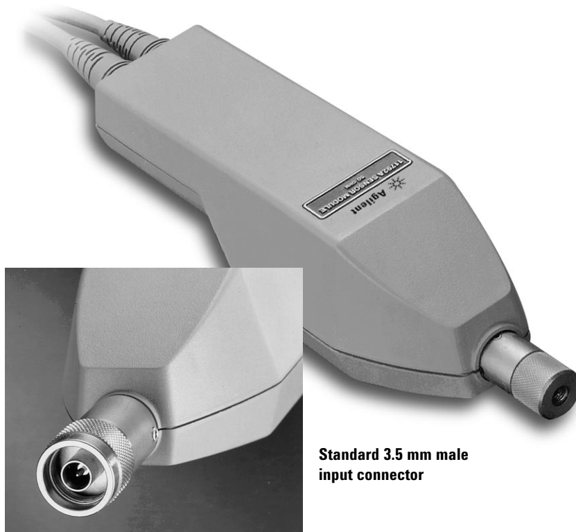
Option 001 N-type male input connector (frequency range to 18 GHz)
